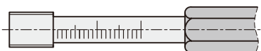
めねじ用(首長ゲージ目盛り付き) For female thread (Neck length gauge with scale)
