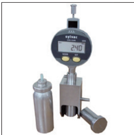
Checking of an internal \varnothing with a mechanical device
