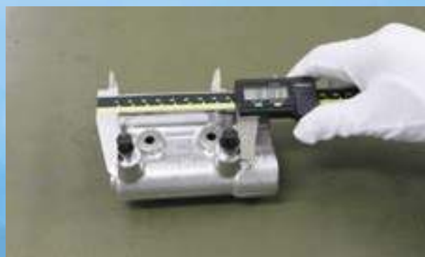
複数のねじ穴ピッチ距離の測定（ノギス測定） For measuring the distance between threaded holes (using vernier caliper)
