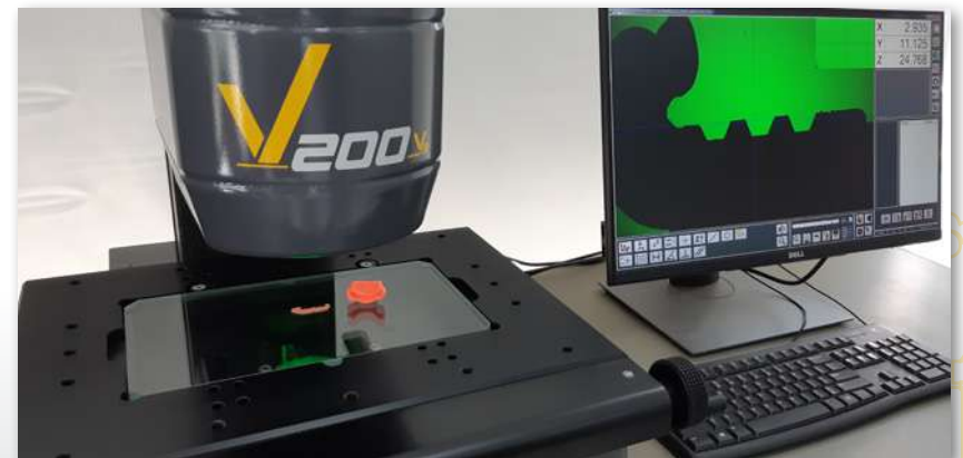
Measure of the flat replica on our VISIO machine
