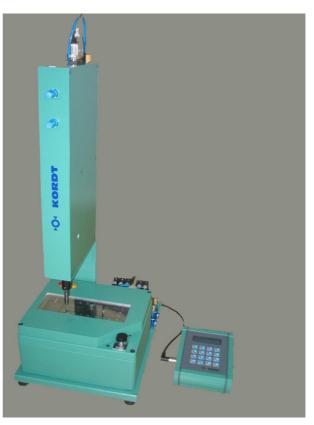
unit have to be applied according to the specifications. Test sequences are started by an external start signal and run automatically. All messages and test results are distributed to the interface.
