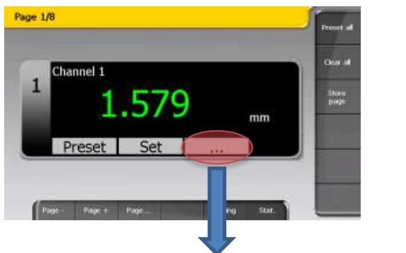
To do this, use the « ... » button (also accessible through the **Setting → Measurement Setting** menu).
