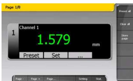
At present, channel 1 is configured to display the A+B value of the two selected instruments and the colour indicates the measurement's status (according to the entered tolerances).
