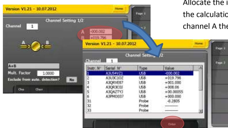
Allocate the instruments to be used to carry out the calculation. Select the instruments for channel A then channel B.
